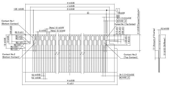
Note: Show recommended dimension when lead for plating is required.
