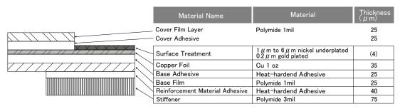
Note 1: This is a reference specification for the FH79 Series FPC construction (t=0.2  $\pm$  0.02mm). The thickness of the FPC mated portion should be 0.2  $\pm$  0.02mm in reference to the construction materials.
