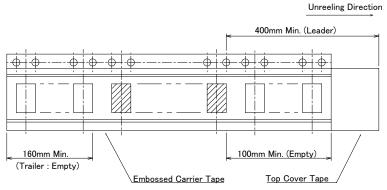
This packaging meets JIS C 0806 and IEC 60286-3 (Packaging of Components for Automatic Handling) standards.
