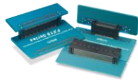
FX18 PCIe Gen.4 (16Gbps) Pitch: 0.8mm No. of Pos.: 40-140 Rated Current: Signal: 0.5A Power: 3A
